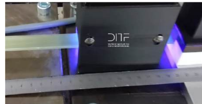
DITF-UV-Pultrusion saves 50% Energy
