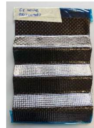
98,19 % of curing rate before pressing
