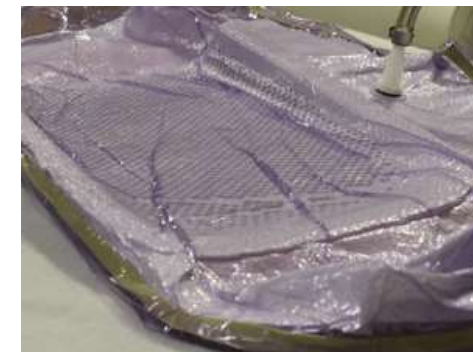
Vacuum bagging of prepreg lay-up
