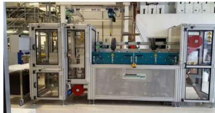
BC 54 impregnation machine from Coatema
