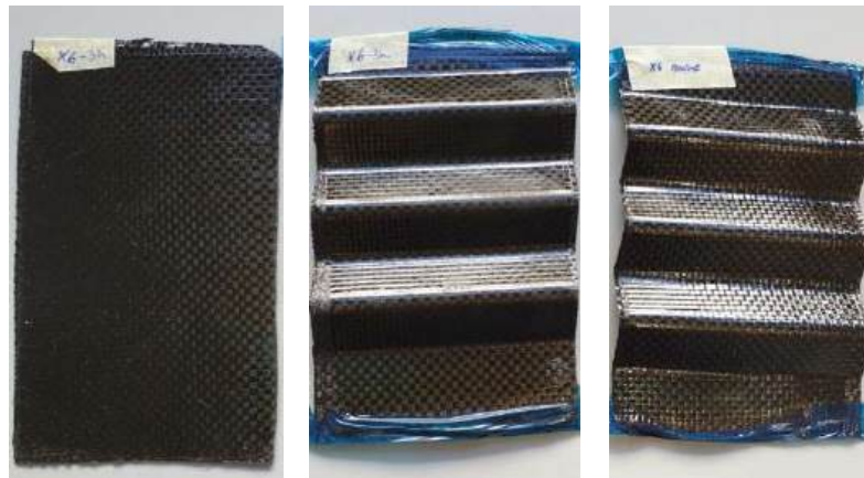
58,98 % of curing rate before pressing
