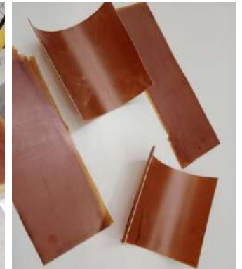
Flat and curved laminate samples, after trimming
