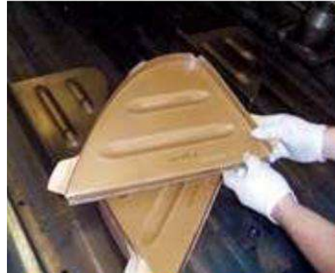
Thermoformed rib (left) being welded to the leading edge skin (right) of the A380
