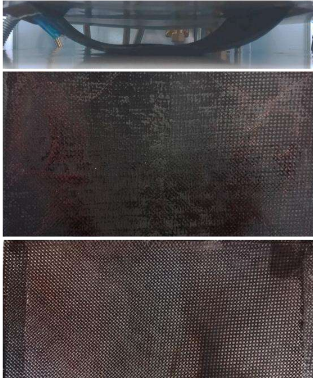
In-plane shear strength testing acc. to DIN EN ISO 14129
