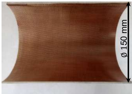
Initial curved laminate, after aging
