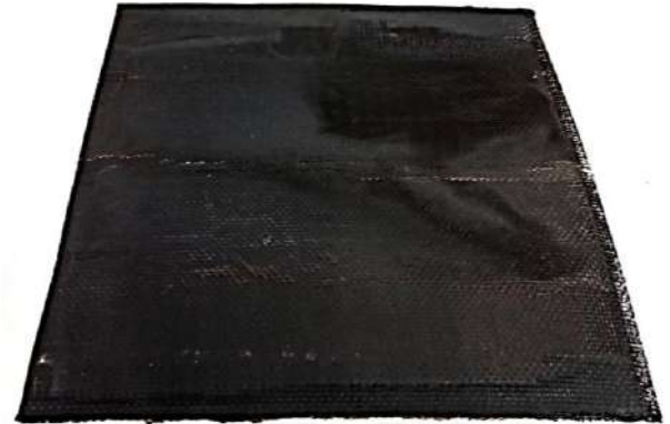
Aged and flattened laminate
