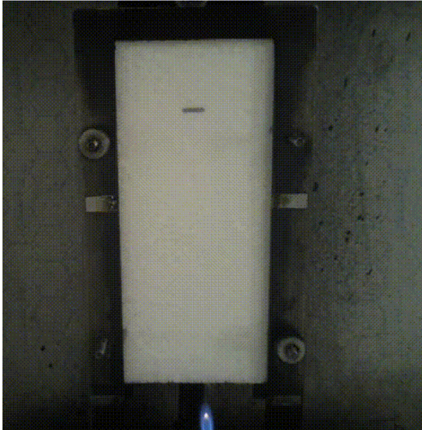
Class E without flame retardant (5 cm and 33 kg/m 3 )
