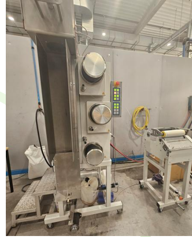
Lab-scale melt extrusion line for multifilaments
