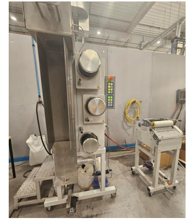
Lab-scale melt extrusion line for multifilaments
